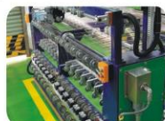
电刷式高压针孔检测安装 electric brush high voltage pinhole inspection installation
